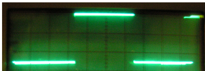
Flipflop output. Verticaal 2V/div
